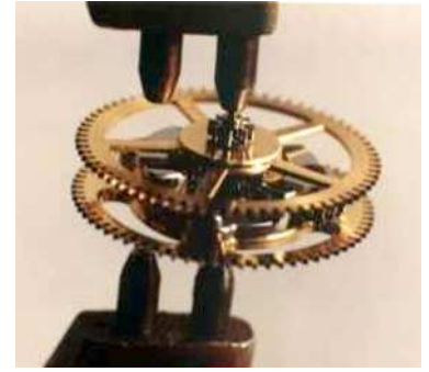
The Differential used in the "Duality" watches "Simplicity" a manual wind without complications.
