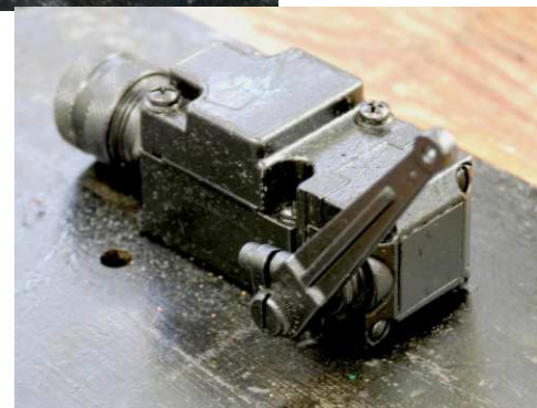
Limit switch after painting and dobbling.
