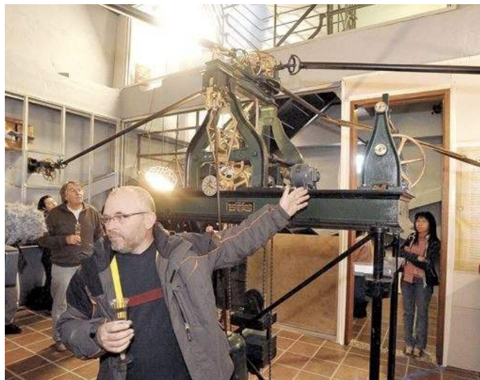
The above photo shows the time train reassembled and back in operating order. The lead off rods are connected to the four motion works. Next comes the chime and strike trains. The aluminum frames along the walls will support the painted murals.
