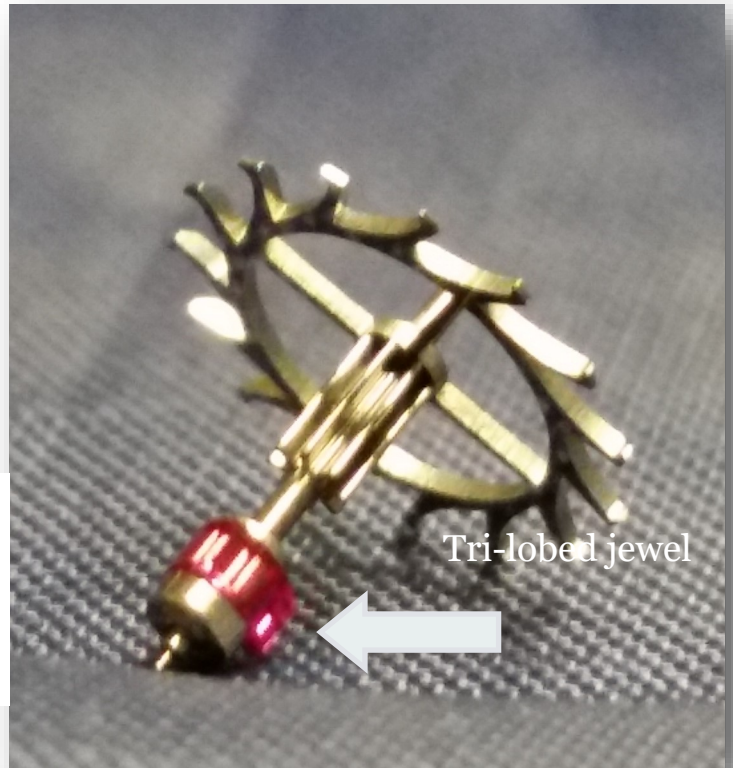
Tri-lobed jewel mounted to escape wheel shaft
