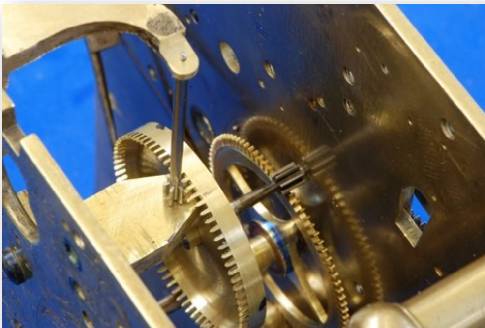
This photo shows the center wheel, the contrate wheel, and the crown wheel arbor in place with top and bottom potences for testing the depthing
