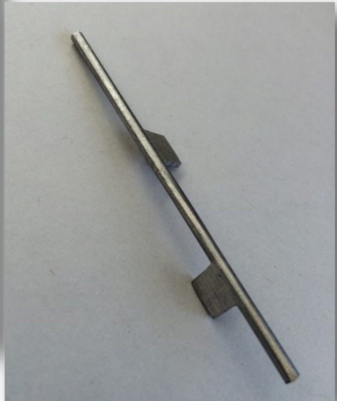
The pallets are cut in half lengthwise, to get their faces in line with the arbor center, and then twisted to get the right offset angle
