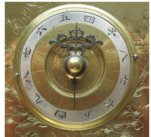
The hand is fixed, and the dial rotates
