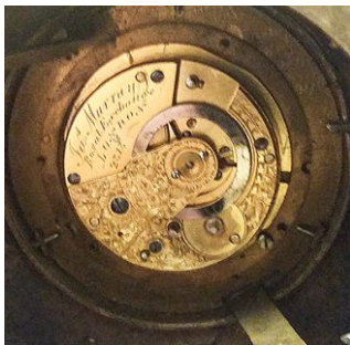
The clock is driven by a fusee watch movement
