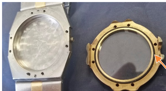
One piece case. Screws attach bezel, with crystal, and seal to the case.
