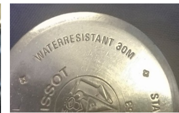
One piece case. Screws attach bezel, with crystal, and seal to the case.
