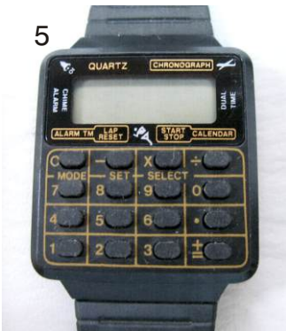
5. Multi-function inexpensive Chinese made wristwatch with a calculator; in a plastic case.
