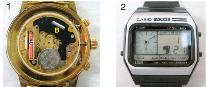
1. The inside view. The coil (A) belongs to the stepping motor. The quartz crystal (B) in its small cylinder.
