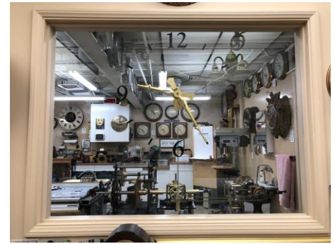
Figure 4. View of the dial, hands and tower clocks from inside the office. The motion works and hands are mounted through a hole in the window. The dial numerals and five minute marks are decals.
