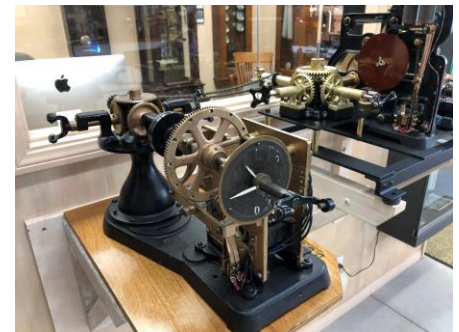
Figure 3. The largest of the two Self Winding Clock Company tower clocks. The cluster gear is driving the clock hands mounted in the window between the office and shop.
