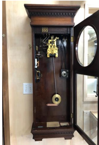
Figure 5. The Self Winding Clock Company master clock with the dial removed showing a myriad of electrical components.
