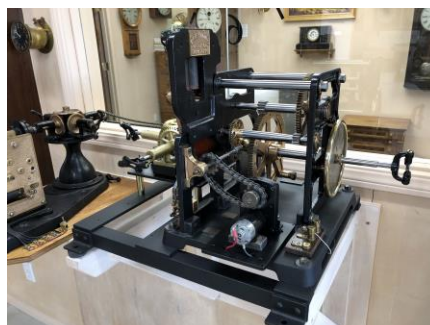
Figure 3. The largest of the two Self Winding Clock Company tower clocks. The cluster gear is driving the clock hands mounted in the window between the office and shop.
