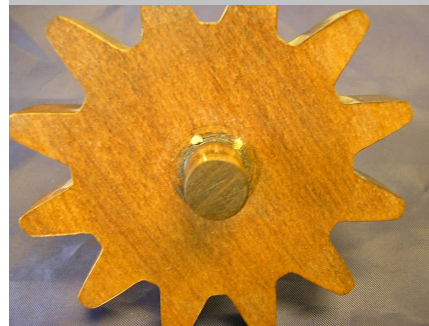
Dowels are trimmed flush with wheel
