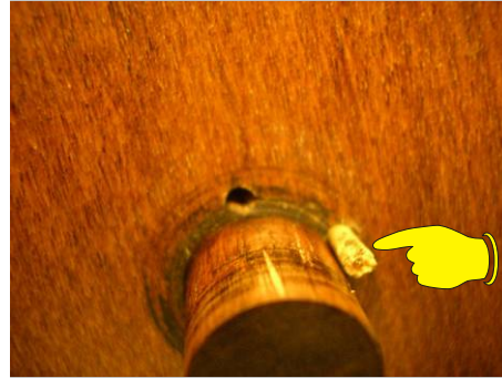
Wheel assembled on arbor and locking dowel inserted.
