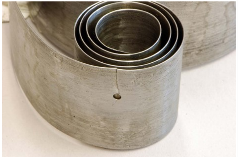
Figure 12 The mainspring from this clock was cracked in two places. A hole had been drilled at the end of the crack in an attempt to prevent further cracking.
