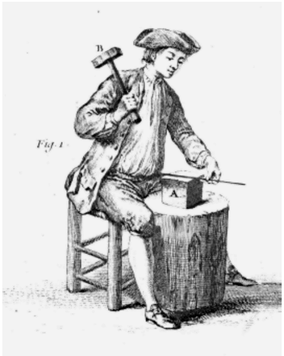
Figure 2 Forging the mainspring (Fig 1, Plate 2, Blakey)
