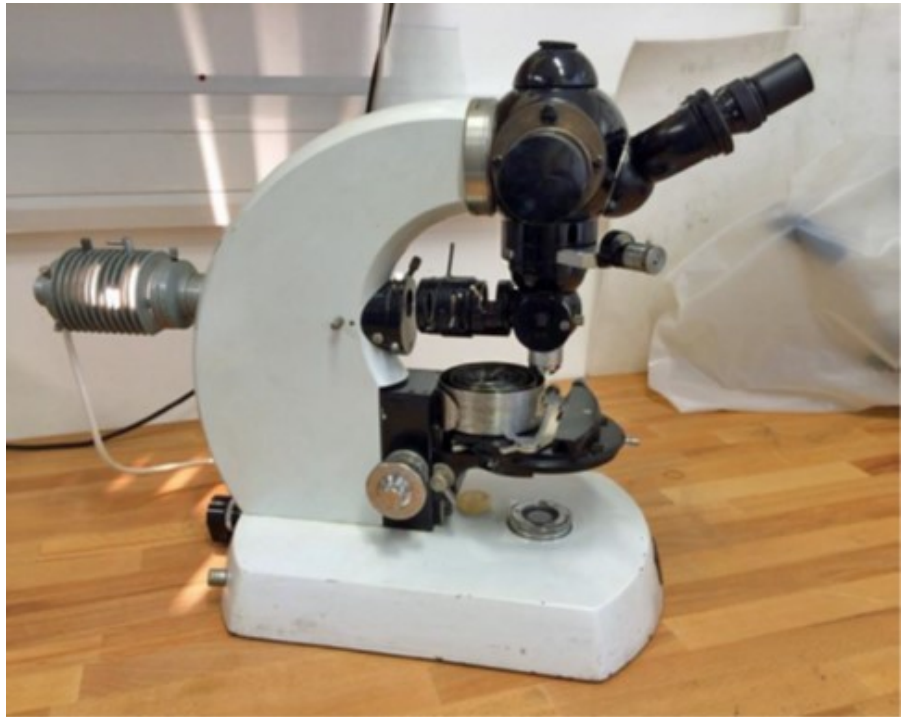
Figure 6 Mainsprings were viewed under 400x power microscope to identify the presence of inclusions
