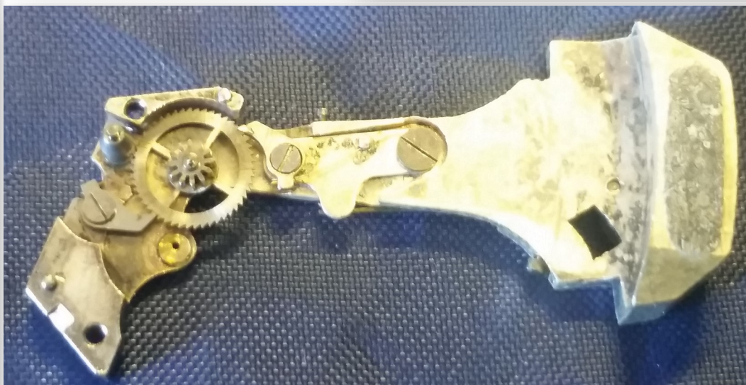
Close up of the automatic winding mechanism and its pendulum/weight.
