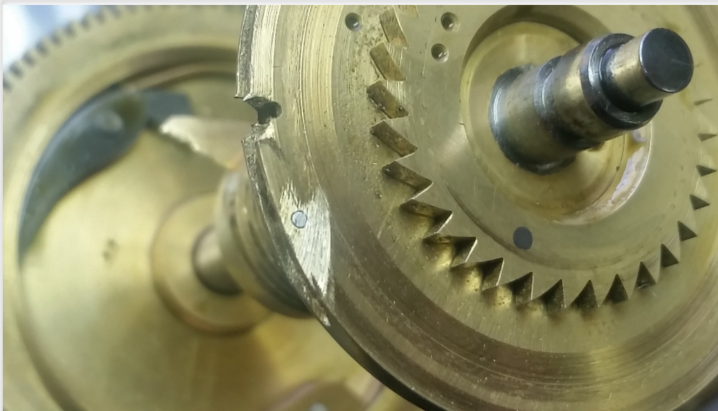
Modification complete showing newly installed anchor pin
