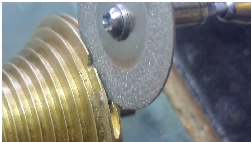
A diamond-impregnated wheel being used to modify the fusee to provide a new anchor point for the hook
