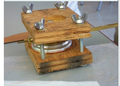
A close-up of the pendulum bob casting fixture
