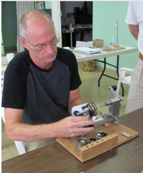
Lex demonstrating the fine art of using the spring winder
