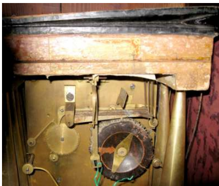
The bellows are on the top, and the wind chest is below them. The round black object is the wood music wheel.
