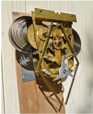
Spring driven "Gravity Escapement" movement, mounted to a board to show how it works.
