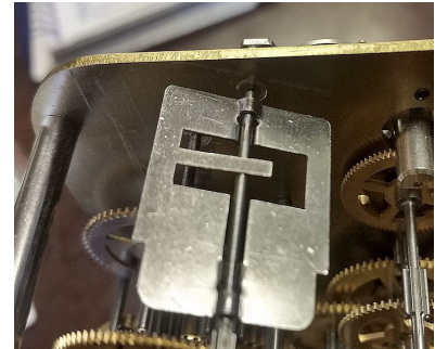
Fig. 1 Steel "finger" friction spring integral to governor
